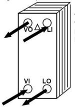
VO = Vapor temperature leaving H/X VI = Vapour temperature entering H/X LI = Liquid temperature entering H/X LO = Sub-cooled liquid leaving H/X
