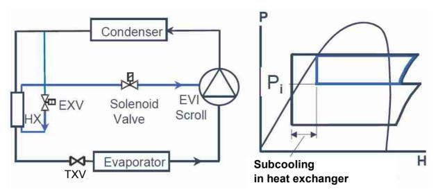
Figure 1-Vapour-injected scroll compressor cycle
